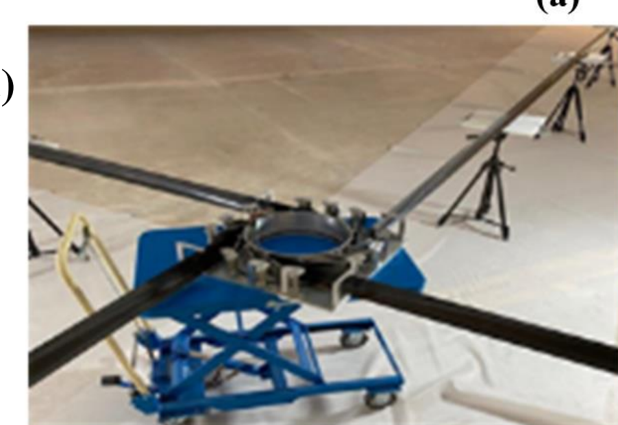
(a) Single deployed quadrant of the Solar Cruiser sail system utilizing 30 m TRAC masts with a side dimension of 40-m. (b) Membrane manufacturing facility at NeXolve which is capable of producing sunshield layers to meet the SALTUS area. (c) A four-mast TRAC deployment system matured to TRL-6. Image credit: NeXolve (a, b), Redwire Space (a, c). Northrop Grumman obtained permission from NeXolve and Redwire Space to include this graphic. See [1].
