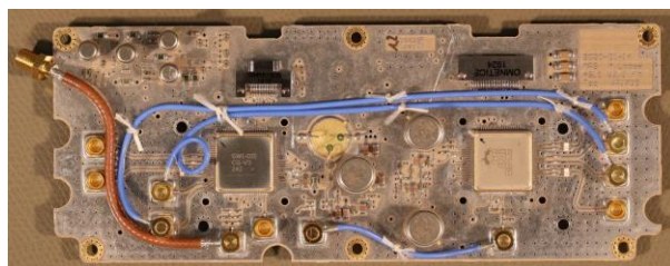
4 5 Fig. 8. ASIC board of SWI-CTS with chirp generator (CGV3) and digital preprocessor (PPV3). [11]
